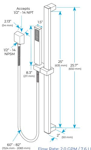
Flow Rate: 2.0 GPM / 7.6 LPM
